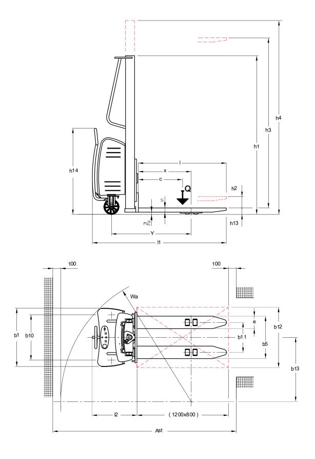
VDI 2198 - Four wheel Forklift Truck top view, reduced load width - b12 / 2 ≤ b13
