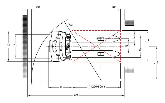
VDI 2198 - Four wheel Forklift Truck top view, reduced load width - b12 / 2 ≤ b13
