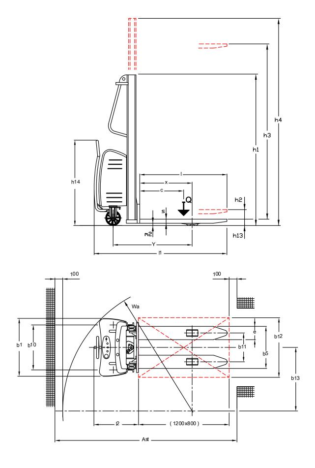
VDI 2198 - Four wheel Forklift Truck top view, reduced load width - b12 / 2 ≤ b13
